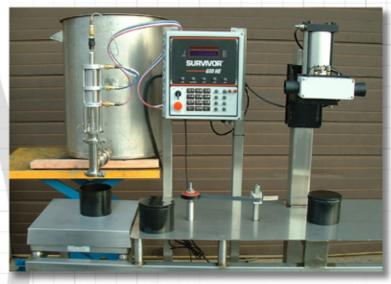
Kinesys Automation's Semi-Automatic Viscous Product/Ink Filling System accommodates a wide range of standard containers including 1/5/10 pound slip-top cans and 1/2/3.5/5/6 gallon containers, and a wide range of cartridges.
