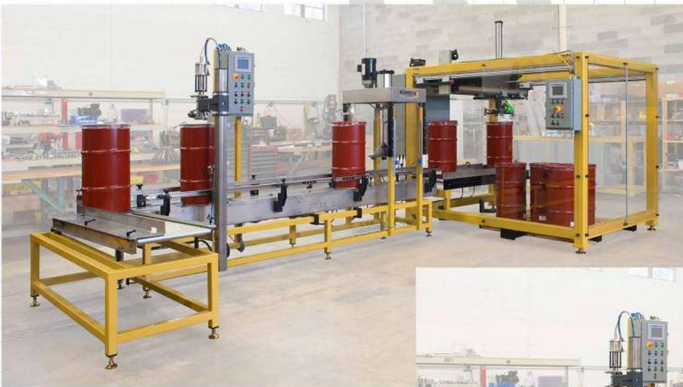
Lid placer is mobile and can be removed or switched out for different style lids. Incorporates quick connect umbilical cables.
