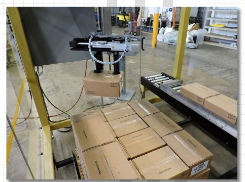
This palletizer is a gantry style, Cartesian robotic system that employs two high-resolution servo motors for xy location with a servo-pneumatic lift cylinder for the z-axis, or three high-resolution servo motors for all three axes. A fourth rotational axis on the pick-up head is available in servo or pneumatic, depending on the application.
