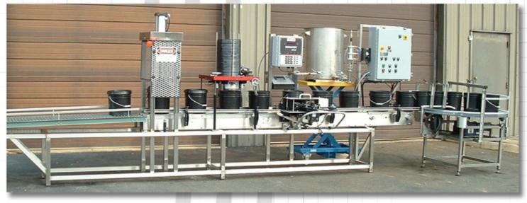
Kinesys' Automation's Automatic Viscous Product/Ink Filling System accommodates a wide range of standard containers including 5/10 pound slip-top cans and 1/2/3.5/5/6 gallon containers.
