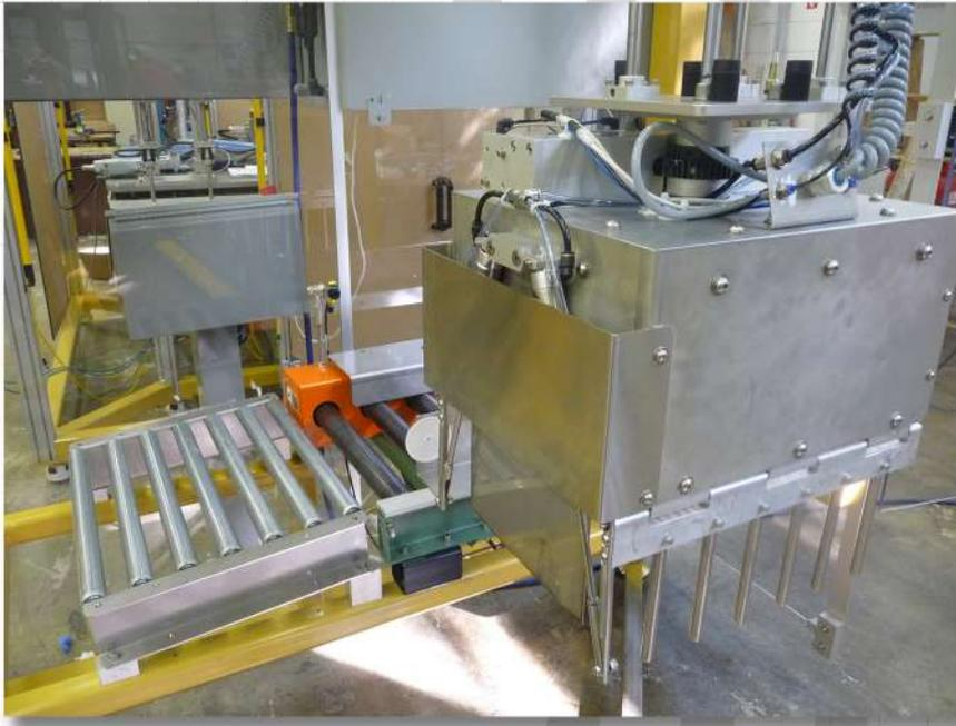
Including a pallet dispenser and pallet conveyors, the system is available as fully automated with empty pallets entering from one side, while completed pallets exit from another side.
