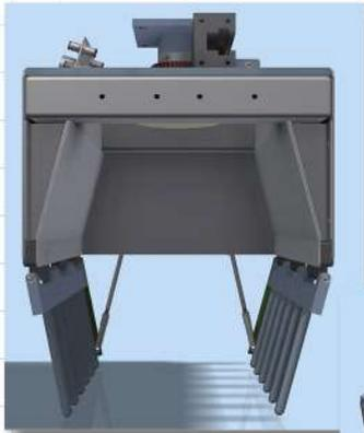
System features a uniquely designed, servo driven or pneumatic, mechanical gripper style bag pick-up head. In the event of power loss or an emergency stop, the pick-up head maintains firm control of the bag thus preventing instances of dropped product.
