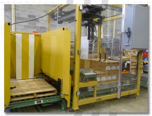
Including a pallet dispenser and pallet conveyors, the system is availaable as fully automated with empty pallets entering from one side, while completed pallets exit from another side.
