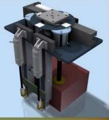
System features a uniquely designed, servo driven or pneumatic, mechanical gripper style case pick-up head. In the event of power loss or an emergency stop, the pick-up head maintains firm control of the case thus preventing insatnces of dropped product.
