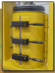
1/4" thick steel reinforced drum shroud.
