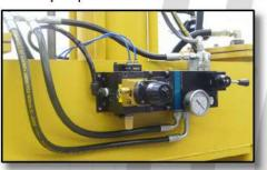
Small package that includes all air and hydraulic gauges, air regulator, exhaust muffler, and all necessary pneumo/hydraulic valving.
