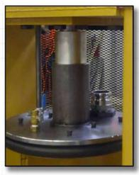
2" thick steel pressure plate with captive 1-1/2" diameter O-ring.
