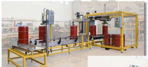
Lid placer is mobile and can be removed or switched out for different style lids. Incorporates quick connect umbilical cables.
