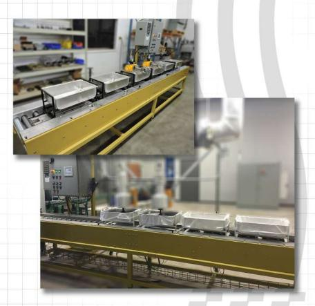
This unique filler uses a combination of powered DC rollers and an indexing beam to move product from one end to another.
