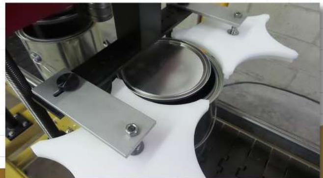
The starwheel alignment fixture ensures that all lids are correctly positioned on the can prior to the lid closing operation.
