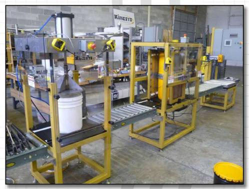
Lid closer with height adjustable, interchangeable heads for plastic press on style lids and metal crimp style lids.
