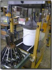
Available with container lifting mechanism for fully-automatic applications.
