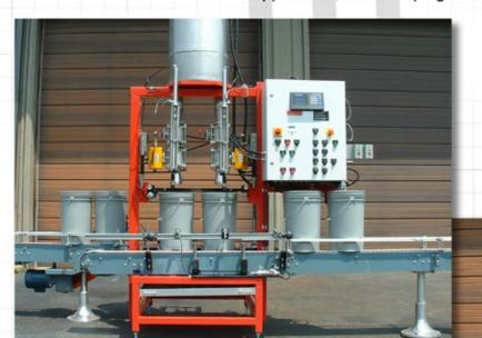
Kinesys Automation's Pail Filling Platform System will accommodate the automated filling of standard 3.5 / 5 / 6 gallon metal and plastic open-top pails via digital netweight fill controls.
