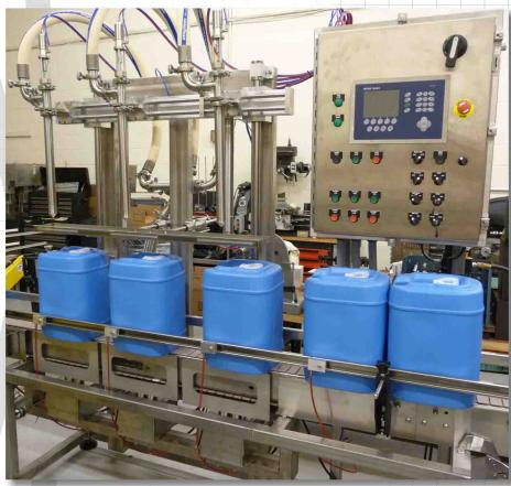
While filling in a gravimetric mode, unique pop up stations housing the load cells raise the container off of the conveyor surface to isolate the product for accurate and repeatable fill weights
