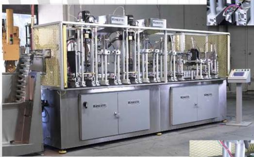
Equipped with dual fillers and dual plunger stations for 2-part cartridge filling and packaging. Universal and interchangeable filler stations with tool less changeover of nozzles for processing any cartridge, regardless of cartridge construction, material volume and viscosity, and size.
