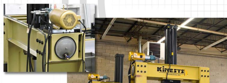
Vessels are rolled into the press at floor height and guided into position with reinforced wheel guides. The hydraulically driven elevator platform then raises the vessel to a height that makes it convenient for transfer. Once at the discharge height, support pins with interlocking safety switches lock the elevator platform into position and the overhead plate is lowered into the vessel to initiate discharge directly to a filler.
